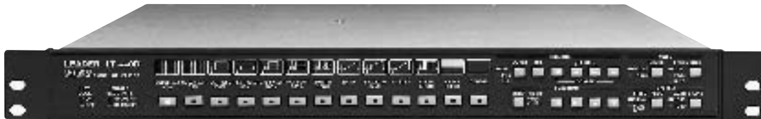
Fig. 11 LT 440D generator. Timing controls are in the GENLOCK group.
