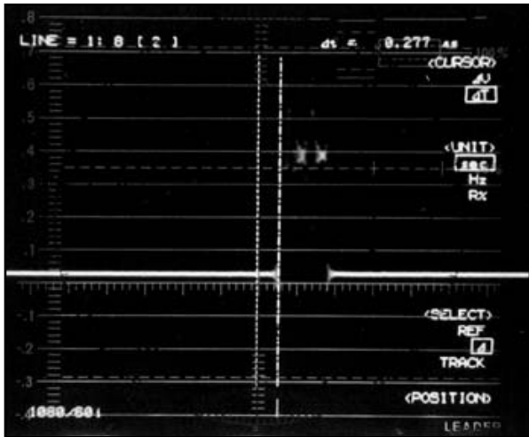
Fig. 6 Small timing error easily corrected with the fine keys. Cursors activated to show the initial error.
