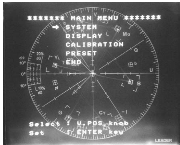
Figure 2-3 Main menu called up by pressing the MENU key allows four choices.
