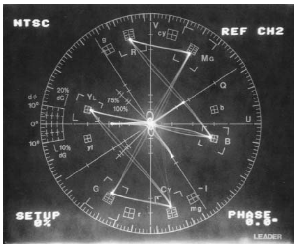
Figure 2-6 Vectors fall short of the targets for SMPTE bars if the vectorscope is calibrated for signals without setup.
