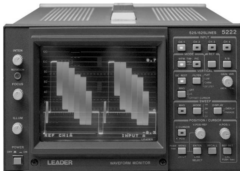
Fig. 1-1 Front panel of Leader's multi-standard 8-channel waveform monitor, Model 5222.
