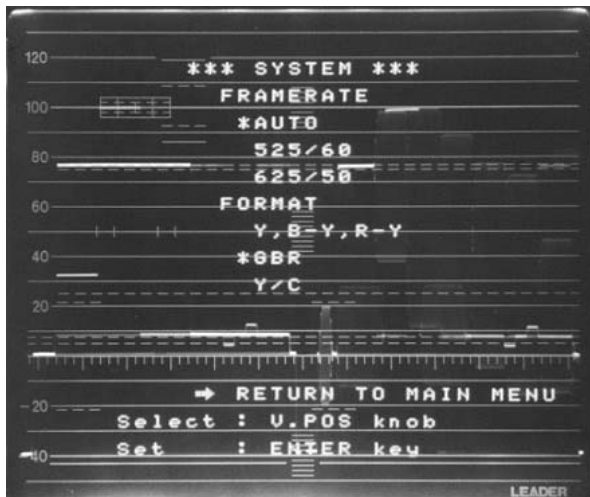
Figure 1-4 System menu. Note that AUTO has been selected for NTSC/PAL/SECAM and that GBR has been chosen for signal FORMAT.
