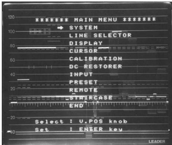
Figure 1-2 Main menu called up by pressing and holding the MENU key for one second.
